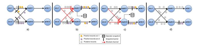
Figure 2: Asynchronous barrier snapshots for acyclic graphs
